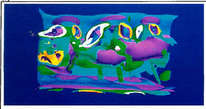
FIGURE 7. Unsteady three-dimensional flow; high-step case (run 3DFSa): (a) t=130H/U_0 ; light blue: vorticity modulus |\underline{\omega}|=1.8U_0/H ; yellow: streamwise vorticity \omega_x=+0.8U_0/H ; green: streamwise vorticity \omega_x=-0.8U_0/H ; (b) t=138H/U_0 ; (c) cross-section in the (y,z) -plane, between the second and the third spanwise vortices in (b); view of the streamwise counter-rotating vortices.
